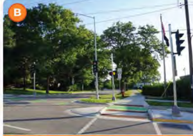
Figure B: Protected bike lanes, pedestrian islands, and bike signals build comfort at Sawyer Terrace and Segoe Road.
