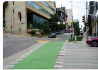
At Wilson, Henry, and Hamilton, raised crossings, pavement markings, and bike signals put cycle track and sidewalk users first.
